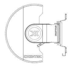
Make sure the kMeter holder has two 1.5 volt AA batteries inserted before attaching it to the kPulley Go.
